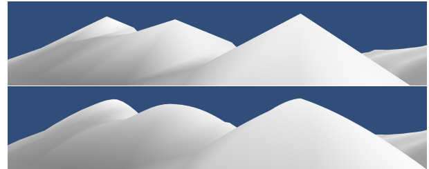
Figure 3: Terrain rendered without (top) and with (bottom) phong tessellation. Notice how sharp peaks are successfully minimized.
